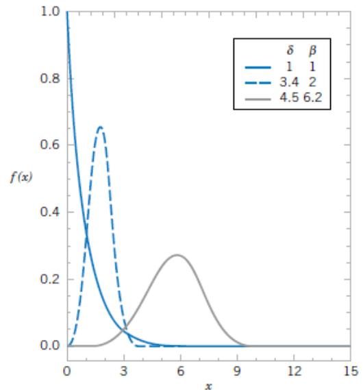
Figure 4-27 Weibull probability density functions for selected values of  $\delta$  and  $\beta$ .
