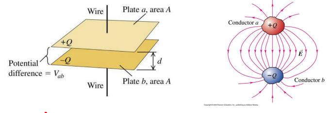
Since there is an electric field between the plates there is also a potential difference between the two plates.
