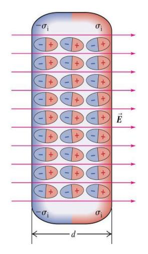
These rearranged charges set up an internal electric field that opposes the electric field due to the charges on the plates
