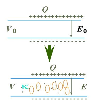
The electric field between the plates of the capacitor is reduced because some of the material within the dielectric rearranges so that their negative charges are oriented towards the positive plate.
