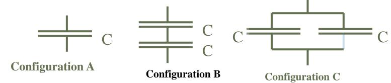
Which of these configurations has the lowest overall capacitance?
