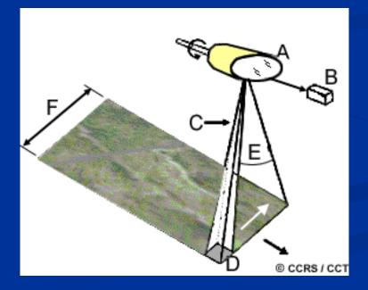
The length of time the IFOV "sees" a ground resolution cell as the rotating mirror scans (called the dwell time), is generally quite short and influences the design of the spatial, spectral, and radiometric resolution of the sensor.
