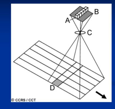
Along-track scanners use the forward motion of the platform to record successive scan lines and build up a two-dimensional image, perpendicular to the flight direction.
