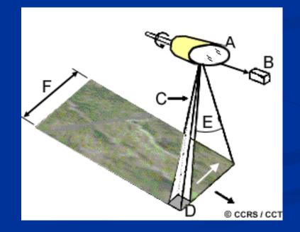
The incoming reflected or emitted radiation is separated into several spectral components that are detected independently.
