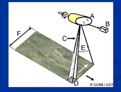
A bank of internal **detectors (B)**, each sensitive to a specific range of wavelengths, detects and measures the energy for each spectral band and then, as an electrical signal, they are converted to digital data and recorded for subsequent computer processing.
