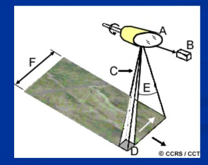
Because the distance from the sensor to the target increases towards the edges of the swath, the ground resolution cells also become larger and introduce geometric distortions to the images.
