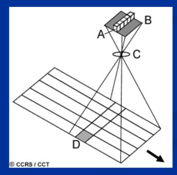
Each individual detector measures the energy for a single ground resolution cell (D) and thus the size and IFOV of the detectors determines the spatial resolution of the system.
