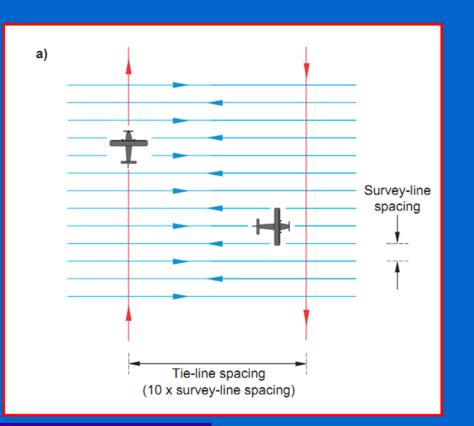
The flight line spacing depend on: Object of survey. Resolution of the data. The cost of the survey.
