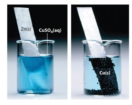
Zn is oxidized and loses electrons to Cu<sup>2+</sup>. To measure the <u>generated electrical energy</u>, we should separate the oxidation from the reduction.
