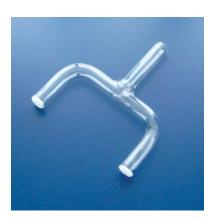
Fill a tube with a viscous aqueous solution of KCl or  $KNO_3$  (using hot agar). The viscosity prevents mixing with the electrolytes. The ions permit exchange of charge.
