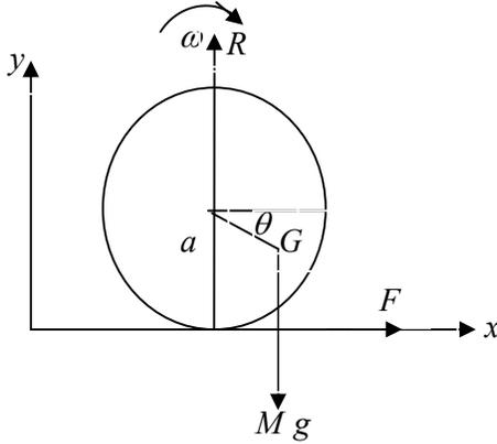
$$\frac{d\dot{\theta}^2}{d\theta} - \frac{2ac \cos \theta}{k^2 + c^2 + a^2 - 2ac \sin \theta} \dot{\theta}^2 = \frac{2gc \cos \theta}{k^2 + c^2 + a^2 - 2ac \sin \theta} \quad (11)$$
