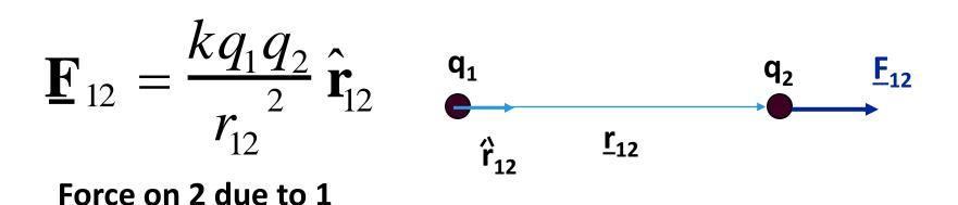
Because the electric force obeys Newton's third law, the electric force exerted by  $q_2$  on  $q_1$  is equal in magnitude to the force exerted by  $q_1$  on  $q_2$  and in the opposite direction; that is,  $\vec{F}_{21} = -\vec{F}_{12}$ .
