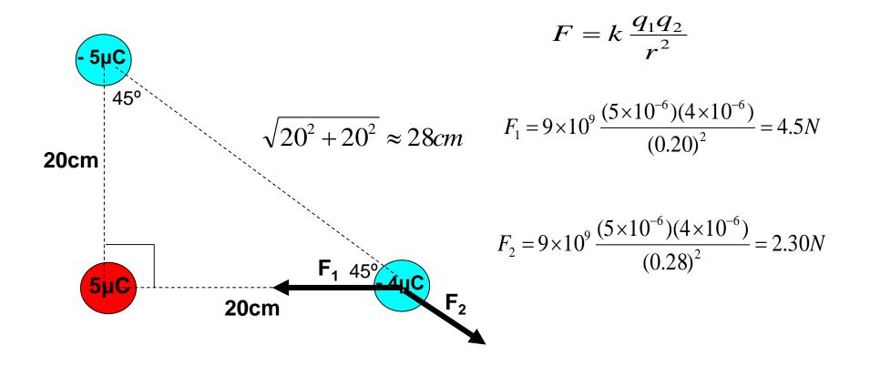
$F_1$  and  $F_2$  must be added together as vectors.
