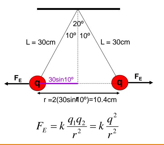
Two identical balls, with mass m and charge q, hang from similar strings of length I.
