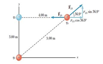
(a) Find the components of the force exerted by  $q_2$  on  $q_3$ . Find the magnitude of  $\vec{F}_{23}$  with Coulomb's law:
