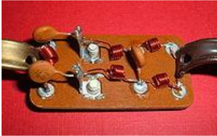
Television signal splitter consisting of a high-pass filter (left) and a low-pass filter (right). The antenna is connected to the screw terminals to the left of center.
