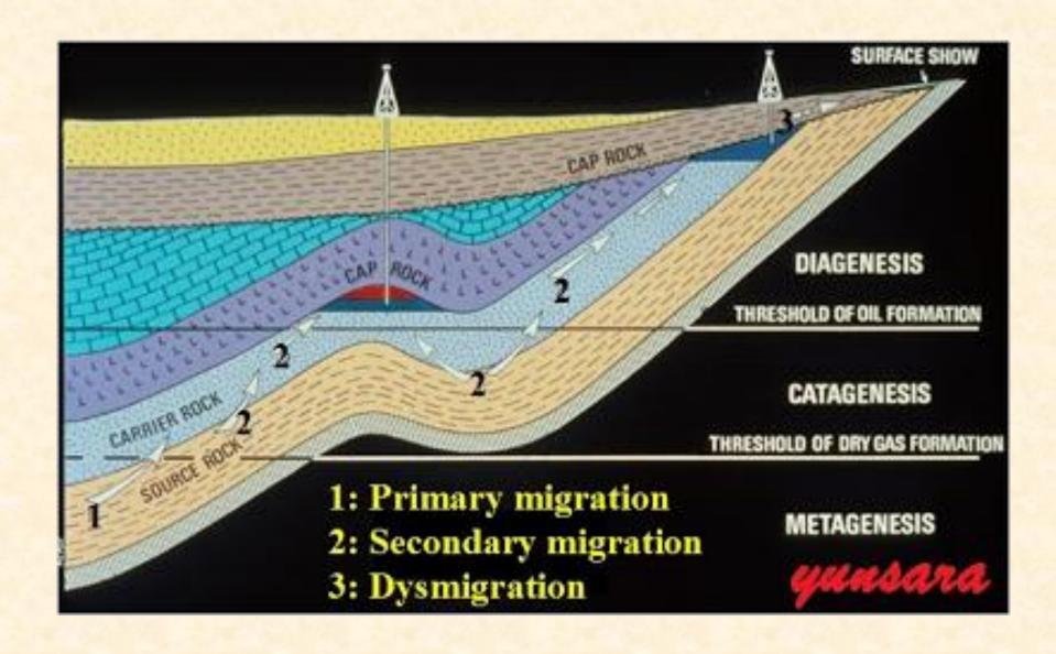
In secondary migration, the oil droplets are moved within the reservoir (carrier bed) to form pools.
